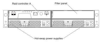
Figure 5. Rear view, single-controller model
